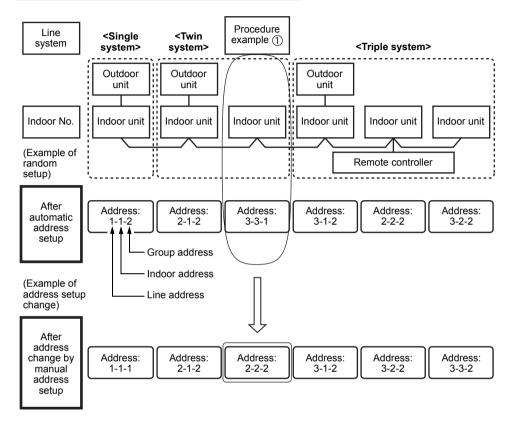
The above address is set by the automatic address setup when the power is turned on. However, line addresses and indoor addresses are set randomly. For this reason, change the setting to match line addresses with indoor addresses.
