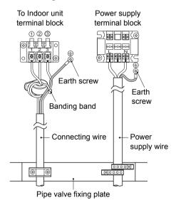
\* Clamp the indoor/outdoor connecting wire ③ and the earth wire together with the ferrite core with the supplied banding band.
