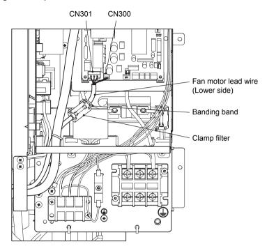
Attach the clamp filter supplied with the outdoor unit to the lower outdoor fan motor lead wire.
