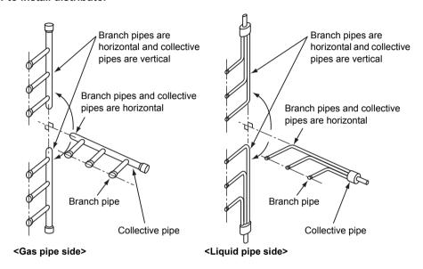
Restrictions in length of the straight area of the branch pipe (main pipe side)
