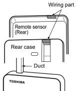
**NOTE 1:**Leave a distance of at least 30 mm around the remote sensor.
