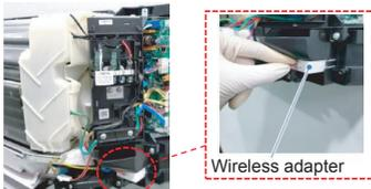
7. Open the cover of Interface Adapter and make hole for wire out.
