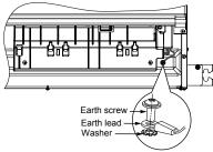
Wiring and connecting cable
