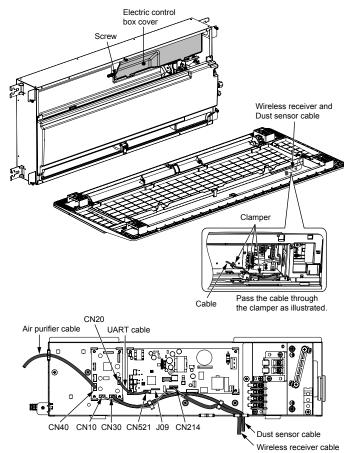
For illustrative purpose the orientation of the indoor unit is not the actual orientation.
