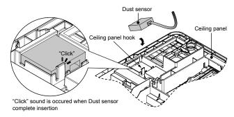
2. Wiring the Dust sensor cable through to the clamp in the back side of the ceiling panel.
